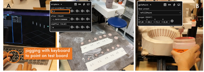
Figure 10: Developing ad-hoc features for the slip deposition machine. A) Making droplets of different sizes on an ad-hoc test plate by triggering extrusion moves of varying length (orange highlight). B) Commanding the syringe to move to the temporary refill station we defined.
