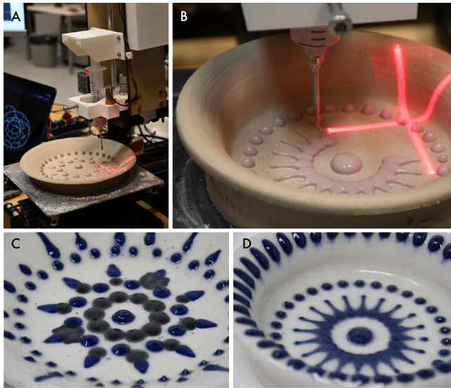
Figure 11: Geometric slip trailing for ceramics decoration. We use the slip deposition machine to deposit droplets of colored slip onto the surface of a thrown plate. A) The machine with a thrown plate. B) The colored slip has to be deposited by bringing the syringe nozzle end close to the surface of the plate. C, D) The decorated plates after firing.
